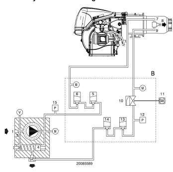
➤ The pump can be considered to be primed when the light oil starts coming out of the screw 4). Close the burner and undo the screws 4).
